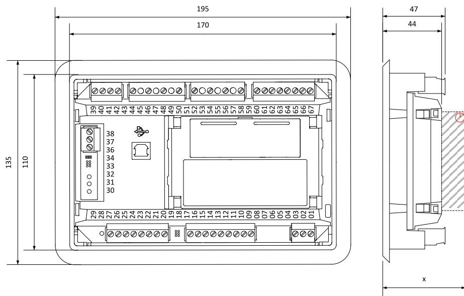
**Note:** The final depth of the controller depends on the selected plug-in module – it can vary between 41 mm and 56 mm. Mind also the size of connectors and cables (e.g. in case of RS232 connector, add about 60 mm more for standard RS232 connector and cable).
