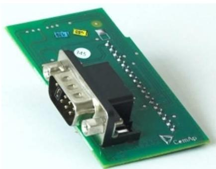
6. Plug RS 232 communication module into the slot of the controller.
