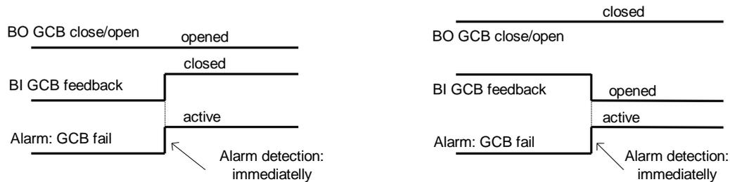
When BO GCB close/open (MCB Close/Open) opens there is 5 sec delay for GCB fail (MCB fail) detection.
